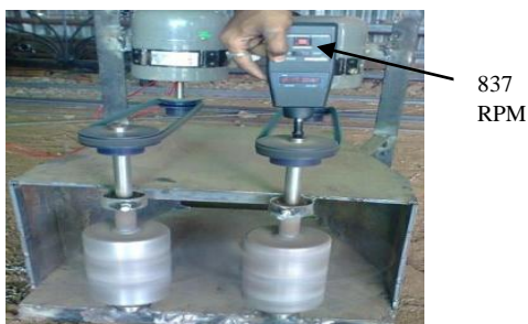
Figure 7. RPM of cutter is measured by using tachometer
